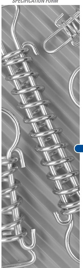
Drawbar Springs are assemblies in which the main spring will compress as the drawbars extend under an applied load. They are often capable of withstanding loads far in excess of the compression springs closing force and should be considered in applications where a positive stop of overload protection is required. Because of the Drawbar Spring's unique characteristic as an extension spring with a fixed stop, potential overstretching is eliminated.
